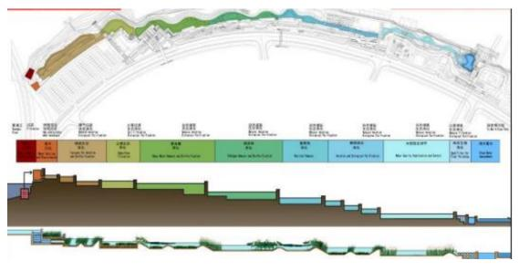
Figure (6) Water treatment in The Park from Lower Grade V to Grade III.
