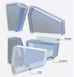
printed three-dimension material. In dependence with digital imitations, the layers classification was taken dimensions before for a thickness of 7 cm (5 cm PCM, 1 cm aerogel and 1 cm container wall thickness). Several samples (17 x 17 x 7 cm) were finished from a numerous of chosen phase changing materials.<sup>xiii</sup>
