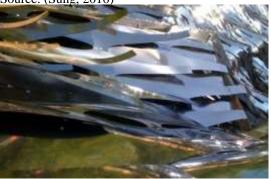
**Fig. 11** A Radial curvature of the thermos-bimetal in a uniform rectilinear shape. Source: (Sung, 2016)
