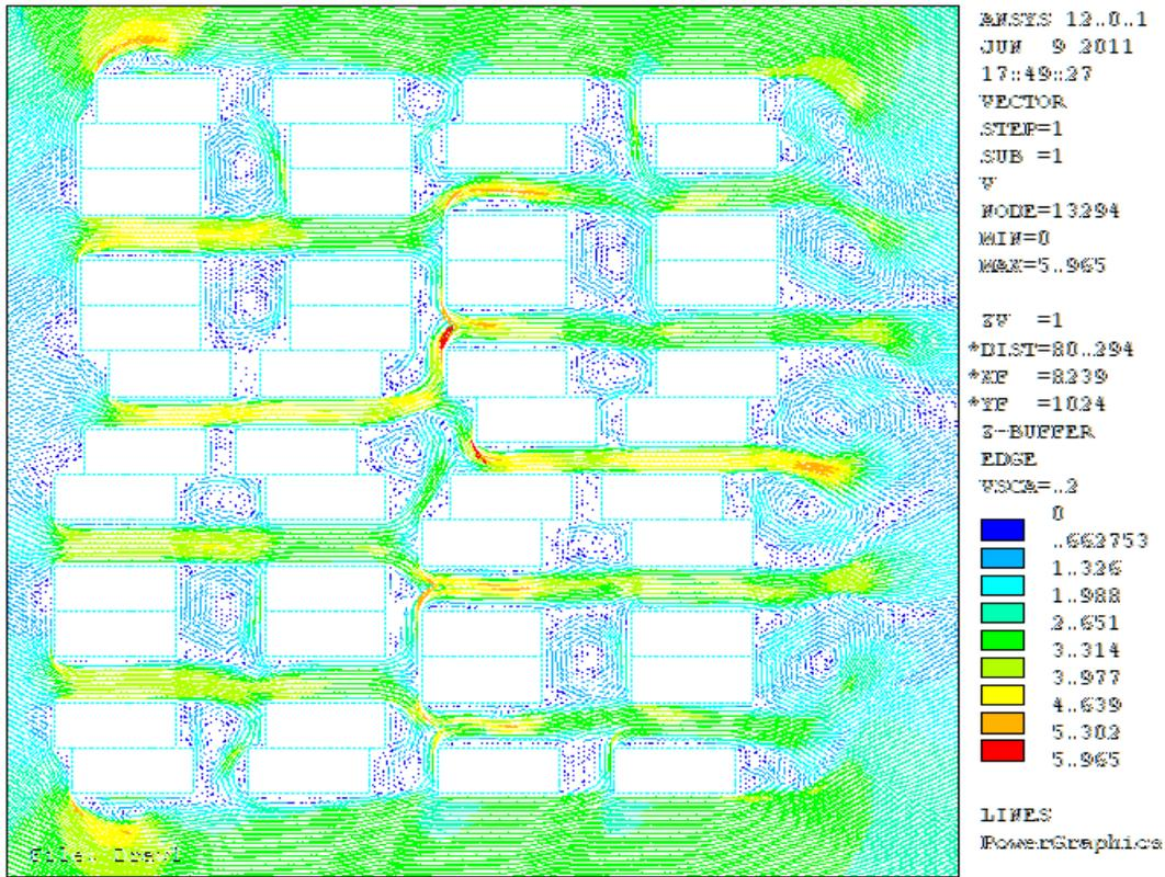
**Fig.5.** Section at streets with ratios and value of air velocity : (A) street that is parallel to wind direction; (B) street is perpendicular to wind (free air velocity 7m/s).
