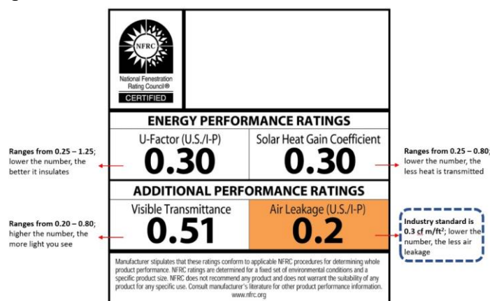
Figure (5). Air infiltration data sheet for the aluminium windows, Source: Ministry of Local Government, 2004.
