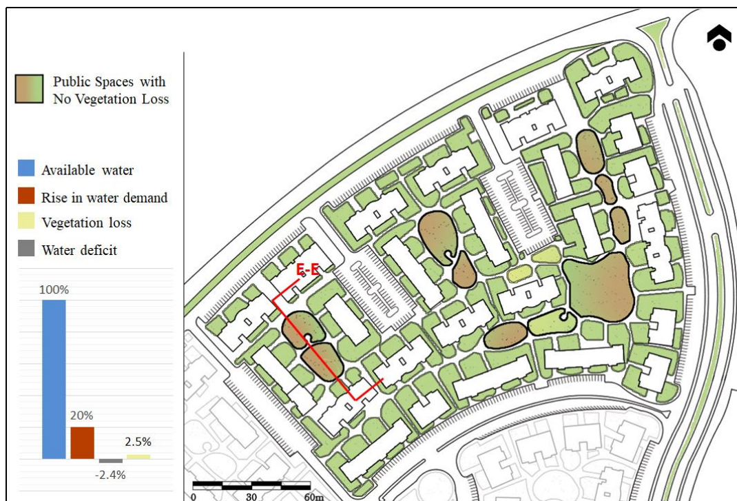
Figure (9). Map of study area 1 showing the open spaces where native plants are proposed, along with vegetation loss results of substituting Bermuda Grass.
