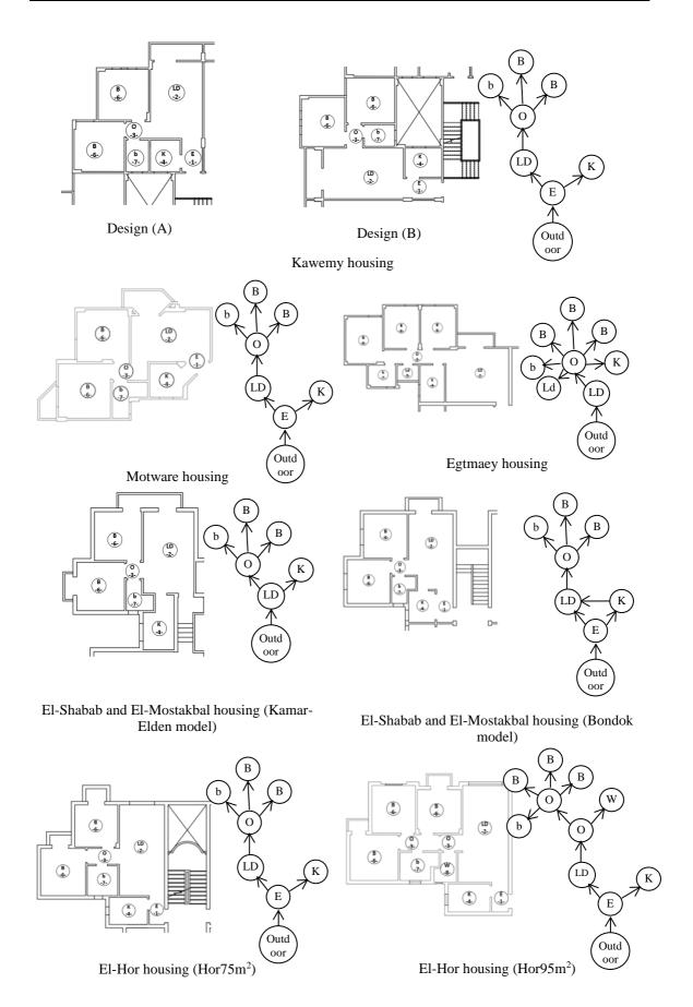
Figure (2). Justified plan graph of the convex spaces. (Source: The author.)
